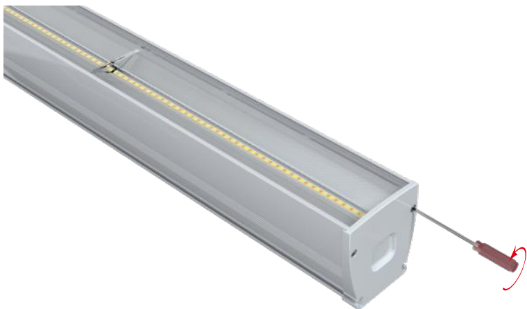
1. Loosen the two screws of the End Cap
