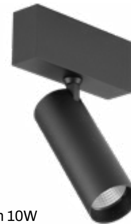
Catania 24Vdc 580lm 8W 2700K RA90 34° Dimmable Low UGR due to dark-light reflectors
